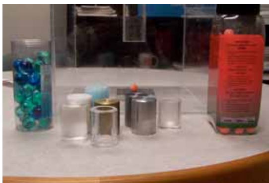
The weights, bath beads, and paints balls used in the splatter box.
